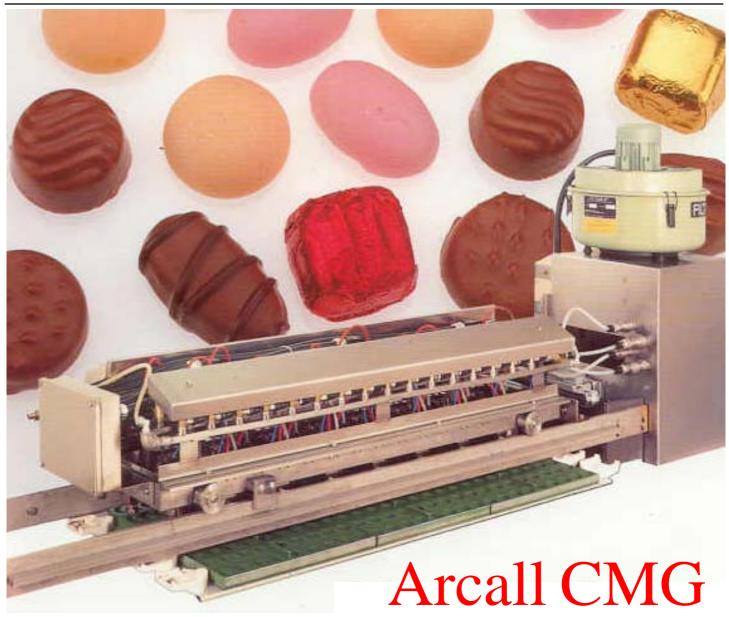
The confectionery mould greaser has been developed to apply a small amount of release agent directly into confectionery moulds. The system sprays accurately into each individual mould and allows considerable product savings. The result is an excellent release, clean moulds and a healthy environment The system is fully food grade with stainless steel spray guns and individual screen plc control on each indent.
